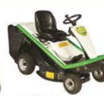
Hydro 80 Kawasaki 16hp 80cm cutting width Optional differential lock
